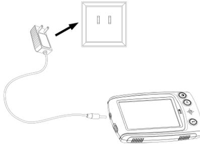
2. When the battery is finished charging, the battery indicator LED will be in green. Unplug the unit. Then the battery indicator LED will turn off.
