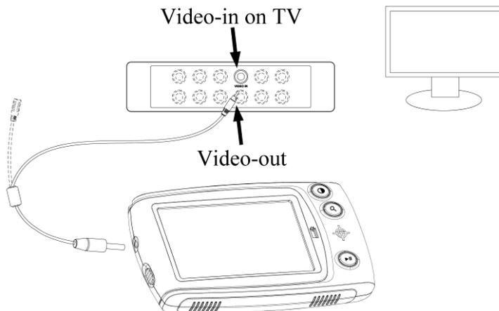
1. Insert the 1/8-inch plug on the end of the supplied Y-shaped video cable into the unit's Power/Video port.
